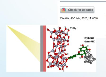
Model systems for dye-sensitized solar cells: cyanidin-silver nanocluster hybrids at TiO<sub>2</sub> support†
