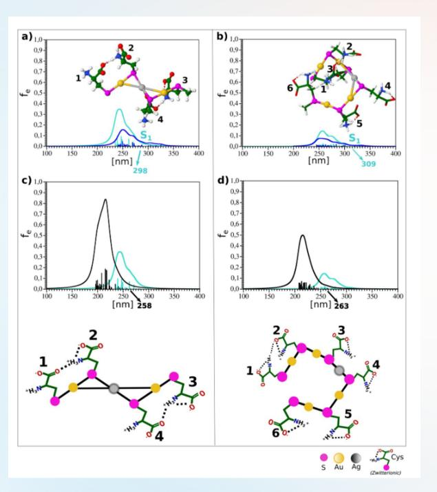
Comparison of OPA spectra obtained for optimized structures of two model systems: a)Au<sub>2</sub>-Ag-Cys<sub>4</sub>-CH<sub>3</sub> and b) Au<sub>4</sub>-Ag-Cys<sub>6</sub>-CH<sub>3</sub> in gas phase (blue) and in water (turquoise) using TDDFT with B3LYP functional and SMD approach for solvent.
